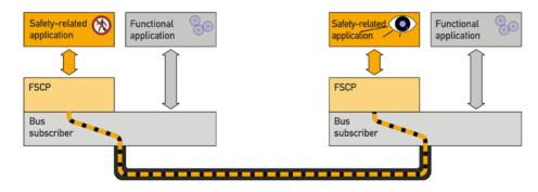
The communication function is generally performed by serial data transmission via a fieldbus (FSCP) or via a point-to-point connection (SDCI). For functionally safe communication via fieldbuses, several profiles have been standardized in the IEC 61784-3-x series.
