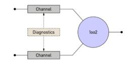
In the machine sector, it is not usual to only output an fault message without changing the output state. Rather, when an fault is detected, the output or outputs are set to the safe state. This is the architecture commonly used so far for the outputs of safety-related devices with a two-channel structure. In the event of a single fault, switch-off of the load is ensured.
