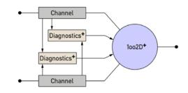
The result of the qualified diagnostics can additionally be made available as a diagnostic status (following Namur NE 131) via status signals:
