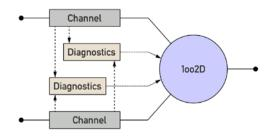
This architecture would allow fault-tolerant continued operation in the event of a single fault in a channel, regardless of the nature of the fault.
