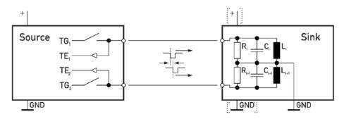
Interface-type C is often used for "OSSD" outputs (Output Signal Switching Device) - e.g. for safety outputs of light curtains.
